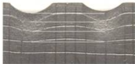
Fig. 1. The grid lines deformation
