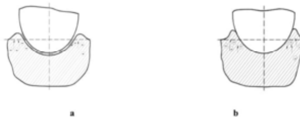
Fig. 4. The scheme of internal stresses' formation: a – lubricated contact; b – dry contact
