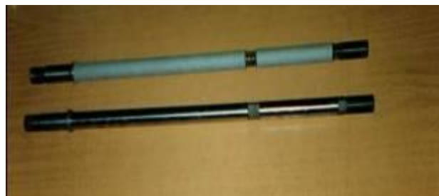
Fig. 7. Compressor piston rod (cylinder 1KU 2GM = 4) with coatings
