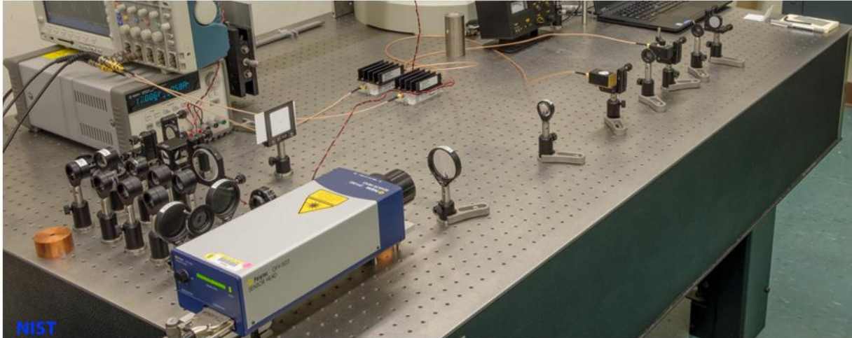
Figure 1: Diagram (upper) and photograph (lower) of the acousto-optic modulator (AOM)-based LDV characterization system.
