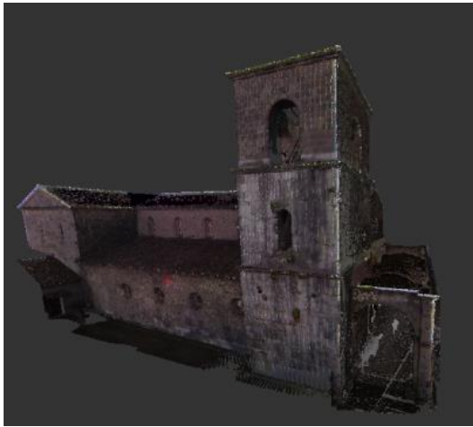
Figure 14. 3D digital model of an external side of the S. Maria della Libera Church.
