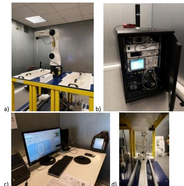
Figure 1. The SATIMO-COMOSAR system used for SAR measurements: (a) COMOSAR test bench and KUKA robot, (b) signal generator Rohde & Schwarz CMU 200, (c) computing unit with OPENSAR software installed for testing system control (d) the fastening system used to secure the measuring equipment.
