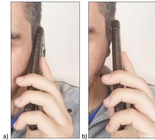
Figure 4. The Huawei P20 Pro phone with a protective case: cheek (a) and tilt (b) position, the two most common positions to the user's cheek.
