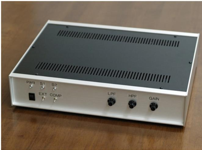
(a) Overview of the developed digital demodulator unit
