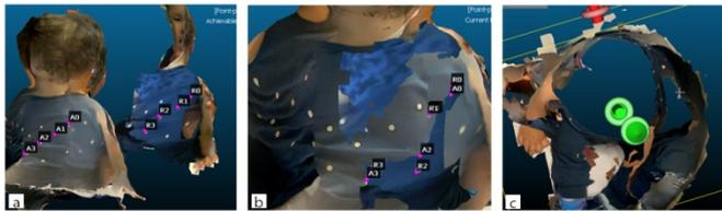
Figure 6. Example of LiDAR scans alignment: a) point selection for alignment; b) alignment; c) top view of alignment.
