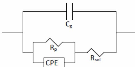
Figure 2. Equivalent circuit used to model the cell solution system to derive the solution resistance  $R_{sol}$ . Electrode polarisation is represented by the CPE element and the polarisation resistance  $R_p$ .  $C_g$  is the geometric capacitance of the electrodes.
