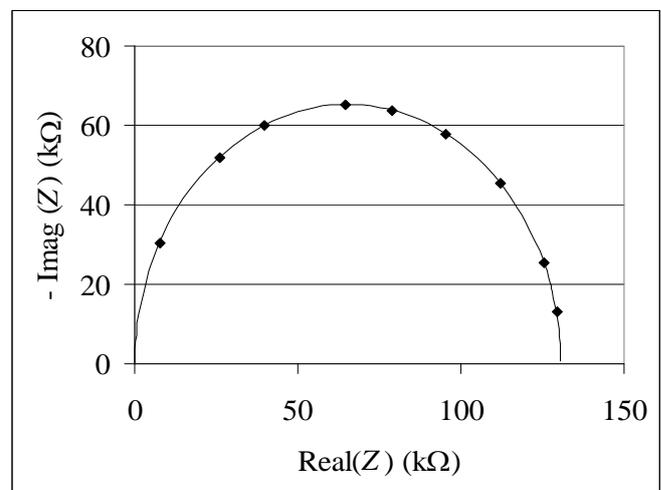
Figure 3. Impedances of a bioethanol sample in a complex plane plot. The dots are the measured impedances  $Z$ , the solid line is a semi circle fit. Frequency range is from 10 to 400 kHz.
