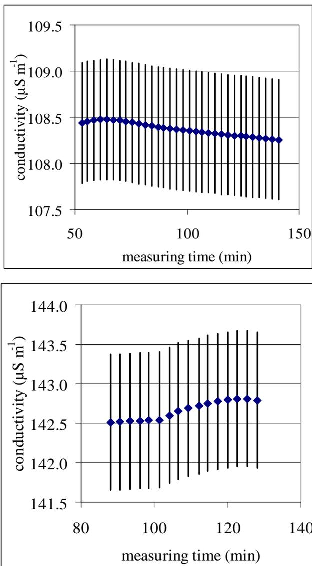
Figure 4. Stability of the conductivity measurement results of bioethanol from Brazil (above) and Germany (below). The error bars indicate the expanded ( $k = 2$ ) uncertainty.
