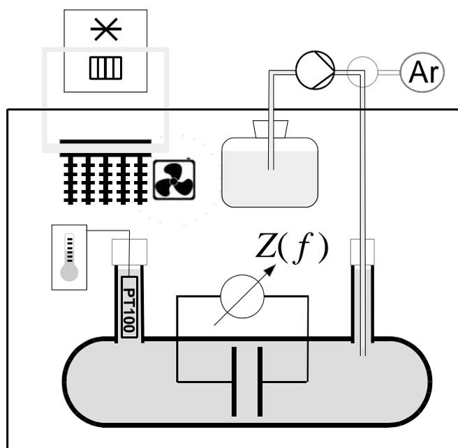
Figure 1. Sketch of the measurement setup, using a two electrode cell that is placed in a temperature controlled air bath. The contact of the sample with ambient air is minimised by pumping it into the cell. Argon is used to dry the cell after cleaning it with ultra pure water.
