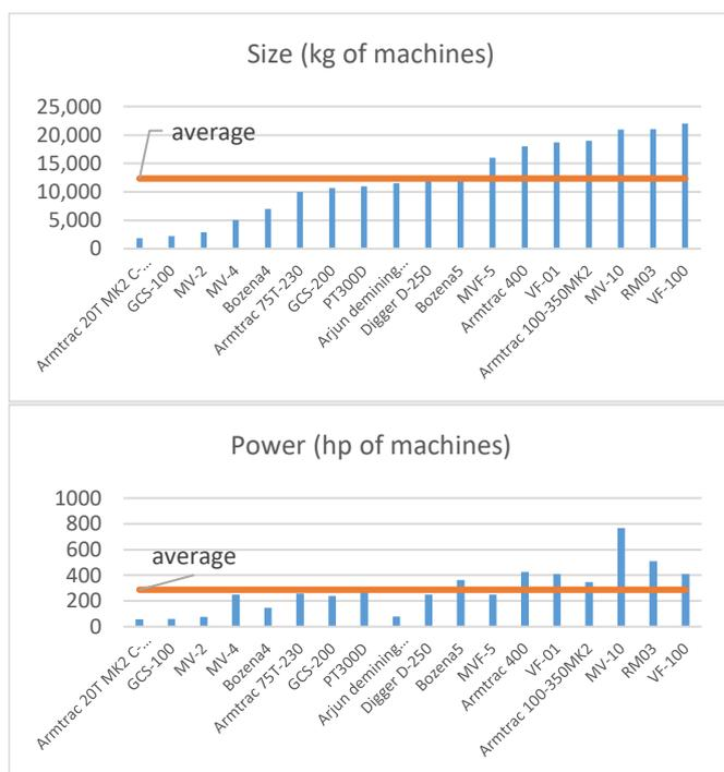
Figure 2. Size (top image) and power (bottom image) of demining machines currently on the market.
