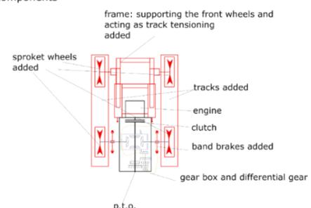
Figure 7. Scheme of Disarmadillo: red parts, frame, wheels, tracks and band brakes are added to the original powertiller (black).
