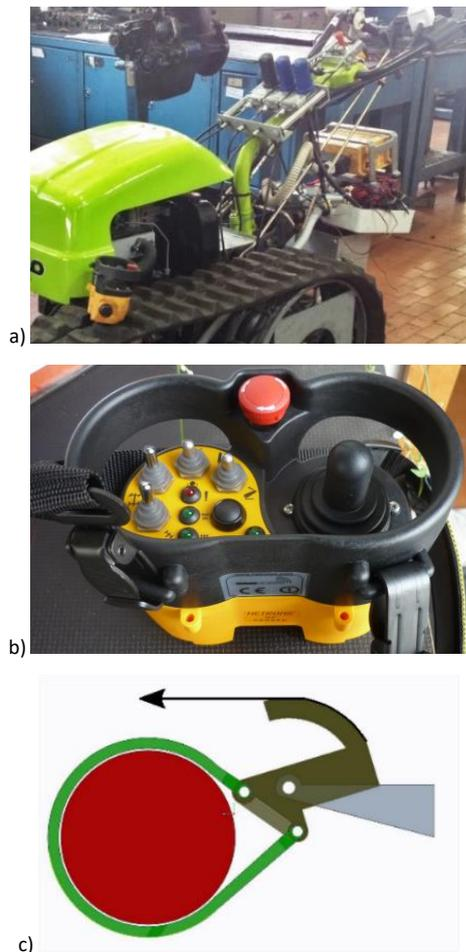
Figure 8. Particular of the control unit: a) linear motors actuating brakes and the clutch, b) transmitter and c) 3D model of band brakes leverage.
