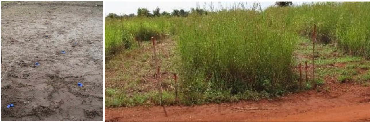
Figure 1. Results from the same demining machine. On the left, test lane used in test site in Germany with dummy Antipersonnel (AP) mines, called WORM, 0 cm – 20 cm deep: 98.22 % neutralized. On the right hand side, suspected hazardous area in Angola: 10 AP mines processed and left live intact (of type POMZ and PP-MI-SR).
