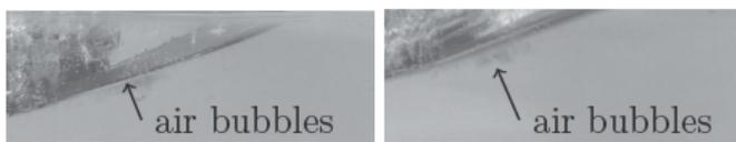
Figure 6. Image of a wedge with deadrise angle of  $15^\circ$  entering the water at 4.2 m/s (left) and 6.7 m/s (right). In both cases there is some air trapped in the fluid in the form of small air bubbles.
