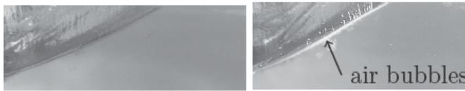
Figure 5. Image of a wedge with deadrise angle of  $20^\circ$  entering the water at 4.2 m/s (left) and 6 m/s (right). There is no air trapped in the case of lower entry velocity while some very small air bubbles appear in the case of larger velocity.
