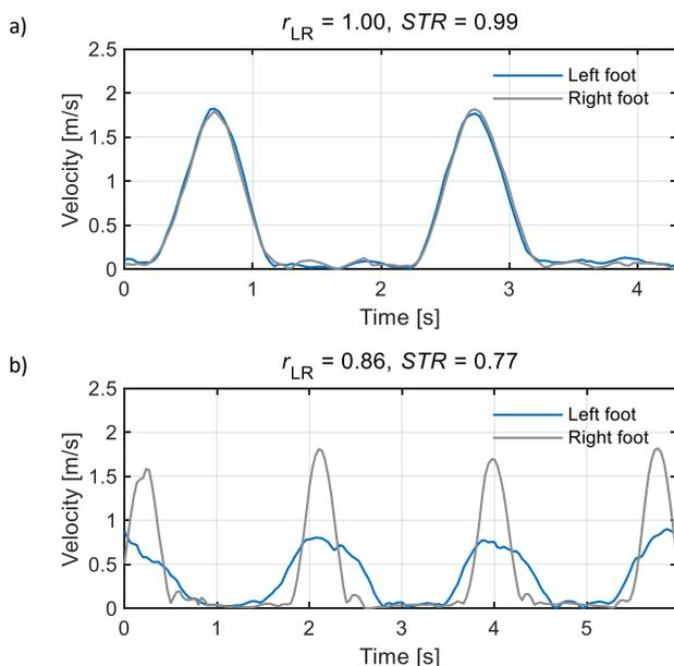
Figure 9. The estimates of the speed of feet, shifted in time so as to maximise the quasi-correlation defined by Equation (1), obtained for quite symmetric gait (a) and quite asymmetric gait (b), and the corresponding values of the indicators of gait asymmetry.
