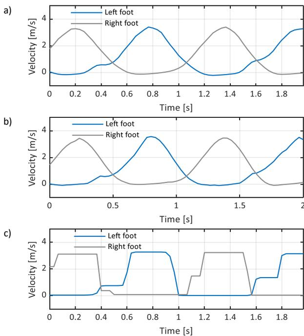
Figure 5. The estimates of the feet velocities, obtained by means of numerical differentiation of some exemplary feet trajectories denoised using the Butterworth filter (a), the Savitzky-Golay filter (b) and the TVR technique (c).
