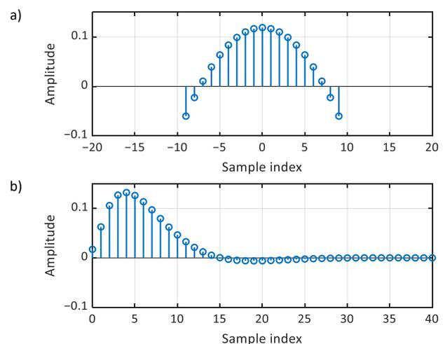
Figure 4. The impulse response of the Savitzky-Golay filter with 19-sample window and 2-degree approximating polynomial (a), and of the Butterworth filter of order 2 with the cut-off frequency 1.4 Hz (b).
