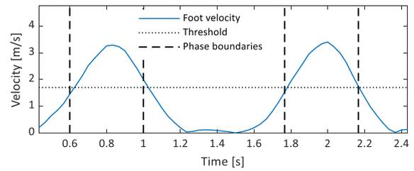
Figure 6. The exemplary results of the identification of the gait-cycle phases by thresholding the estimates of the foot velocity.
