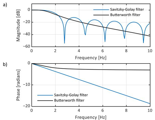
Figure 3. The frequency characteristics of the Savitzky-Golay filter with 19-sample window and 2-degree approximating polynomial, and of the Butterworth filter of order 2 with the cut-off frequency 1.4 Hz.
