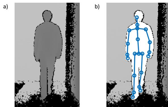
Figure 1. A depth image in which brighter pixels represent larger distance from the sensor (a); a human silhouette, identified in that image by means of the Kinect device (b).
