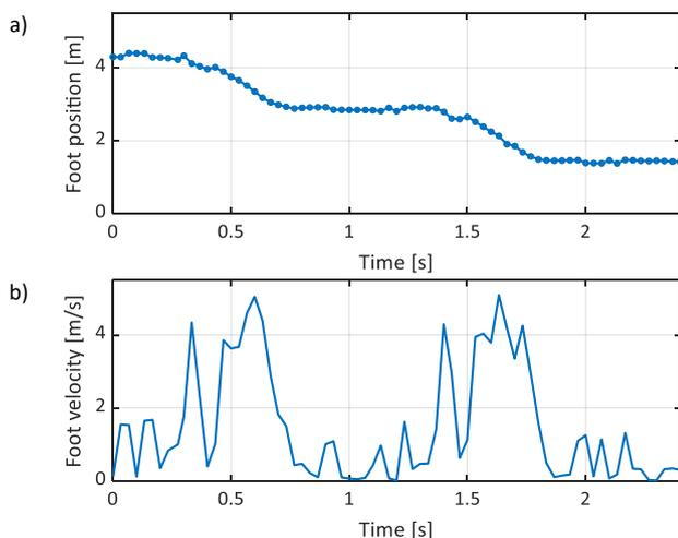
Figure 2. An exemplary sequence of data acquired by means of a Kinect v2 device, representative of the antero-posterior position of the left foot of a person who was walking toward that device (a), and the results of numerical differentiation of that sequence using the central-difference method (b).
