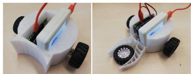
Figure 2. Photographs of different 3D printed robots. In contrast to off-the-shelf robots, the geometry can quickly be adapted to ideally host sensors and actuators. While the left robot can only manipulate objects by shifting them, the robot on the right also includes a simple soft robotics fin ray type gripper [10], which can also be equipped with tactile sensors.
