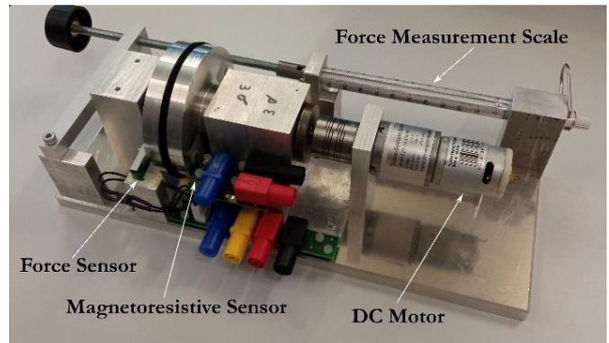
Figure 4. The DC motor has a spinning wheel attached to its shaft. This spinning wheel has holes near its perimeter. The angular velocity of the wheel can be obtained by processing the output signal of the magnetoresistive sensor S1. A brake wheel that can spin freely is mounted next to the spinning wheel, and the force applied can be adjusted and measured. A small extrusion of the brake wheel applies force on the force sensor, whose output can be used to measure the torque.
