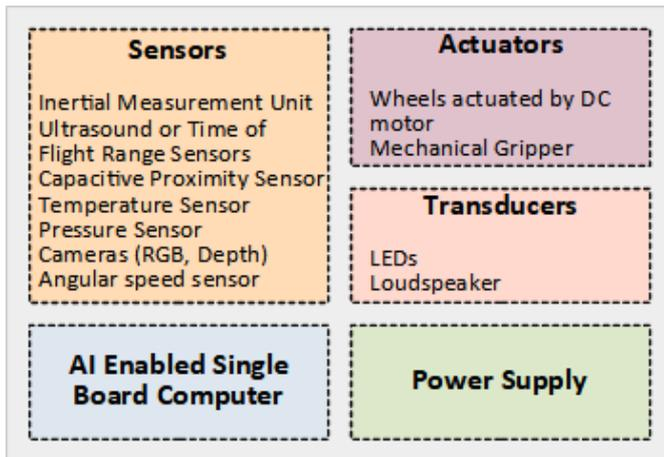
Figure 3. Hardware components in the proposed robotic platform. Depending on the requirements additional components can be included.
