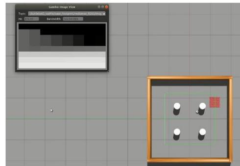
Figure 6. Reinforcement learning with gazebo and time of flight sensors. The aim is that the robot navigates to the red rectangle, while avoiding collisions with the obstacles. The simulated sensor signals are illustrated in the top left image, where the distance is encoded in a gray scale image.
