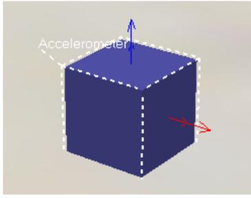
Figure 5. Simple acceleration sensor model in CoppeliaSim®. It comprises an ideal force sensor and a seismic mass, the accelerations are determined by dividing the forces as obtained from the physics simulation engine by the mass.
