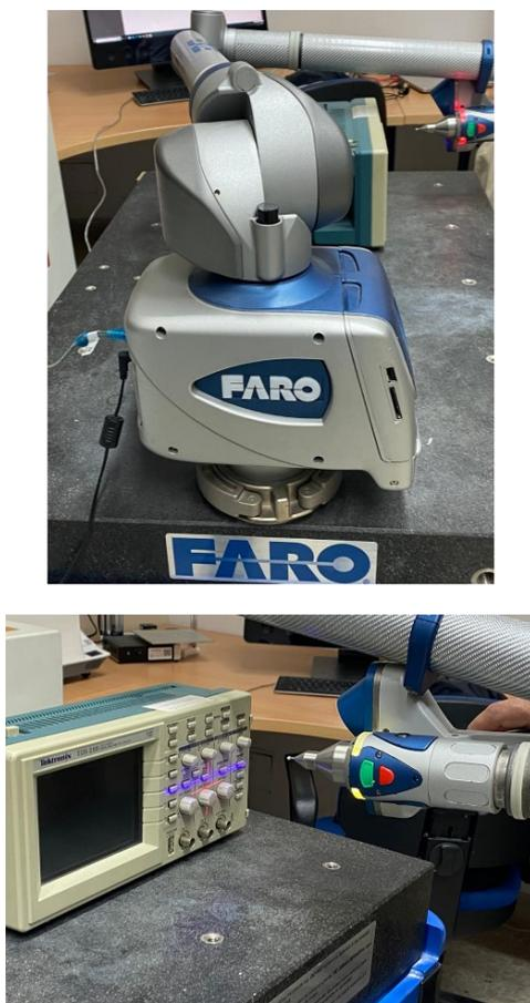
Figure 2. 3D scanning strategy of the instrument exploiting a non-contact Laser ScanArm by FARO™.
