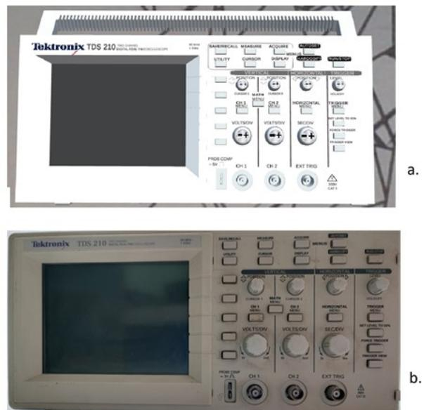
Figure 5. Comparison between the actual instruments and its digital twin; instrument view in the AR software environment (a), actual instrument (b).
