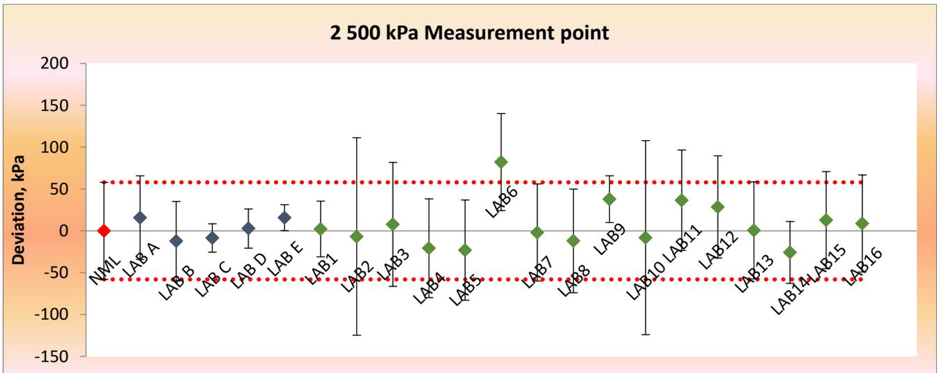
Figure 5. Participant's deviation from the reference values and its corresponding uncertainties at 2500 kPa.
