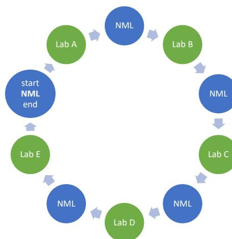
Figure 2. PT 2010 measurement scheme.
