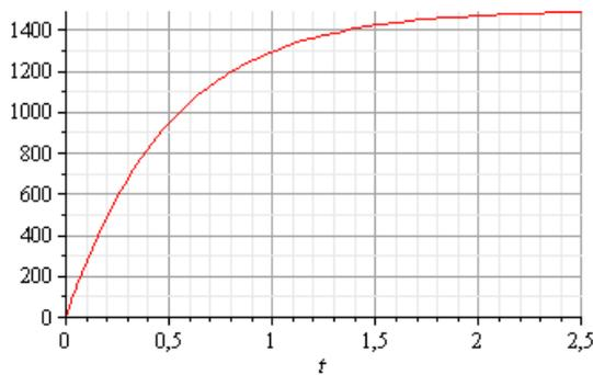
Figure 4. Dependence  $n = (t)$ :  $\tau = 0.5$ ;  $\Omega = 1500$  rpm.
