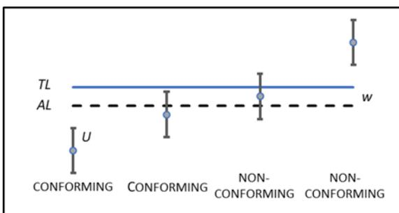
Figure 2. Illustration of the guarded acceptance based on ILAC G8 [1].
