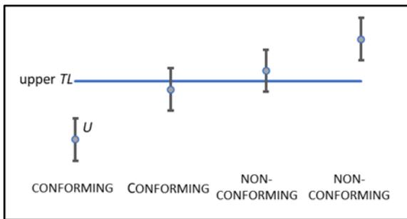
Figure 1. Illustration of the simple acceptance based on ILAC G8 [1].
