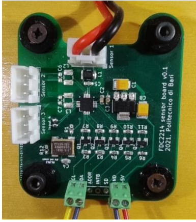
Figure 2. The prototype of the sensor readout electronics based on the FDC2214.
