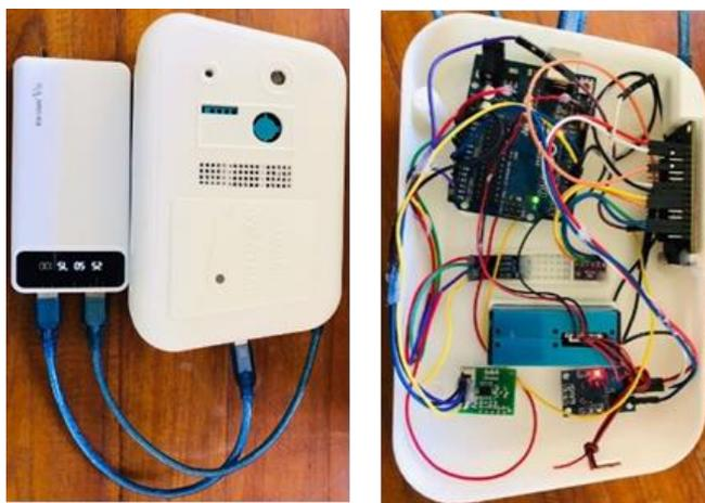
Figure 2. Enclosure and Wiring of the Hardware System includes the sensors AHT10, MQ-07, VOC, BMP280, ESP 8266, PMS5003, ZP07-MP503, and the battery pack unit.
