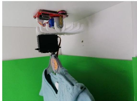
Figure 3. Automatism to rotate the garments.
