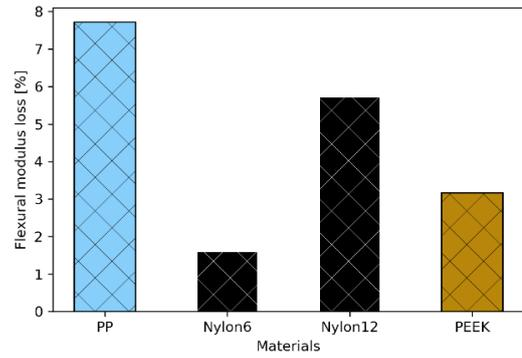
Figure 5. Flexural modulus loss for PP, Nylon6, Nylon12 and PEEK due to saliva exposure.
