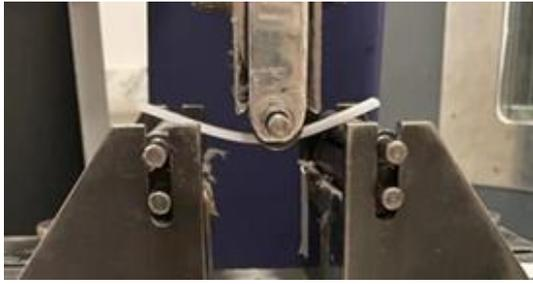
Figure 3. Example of PP sample mounted on the LLOYO flexural strength test machinery.
