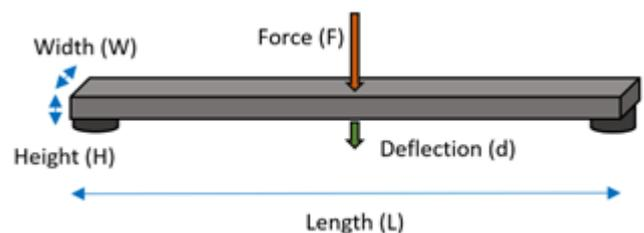
Figure 2. Flexural modulus measurement: 3-point bending test.
