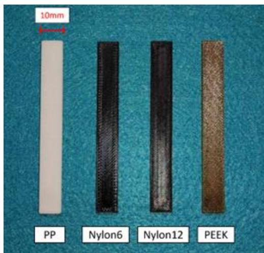
Figure 1. Tested samples materials and geometry.
