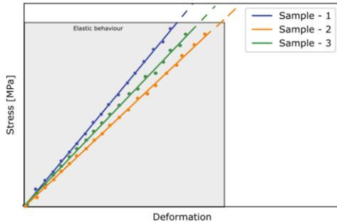
Figure 4. Example of linear interpolation of measured data for a generic material (differences in behavior are enlarged for the sake of comprehensiveness).
