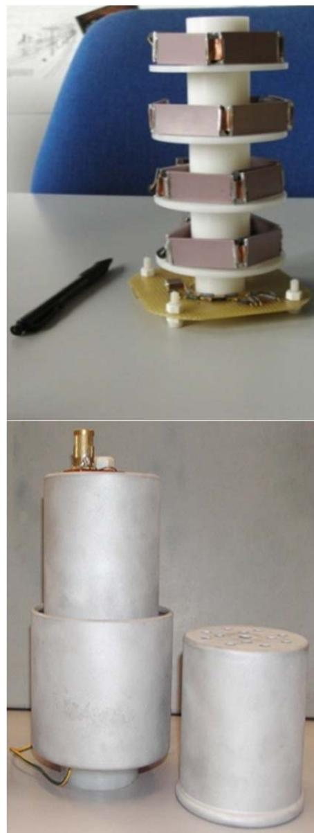
Figure 1. Resistive-capacitive shielded divider during the assembly step.
