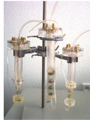
Figure 6. The cells for the primary standard.
