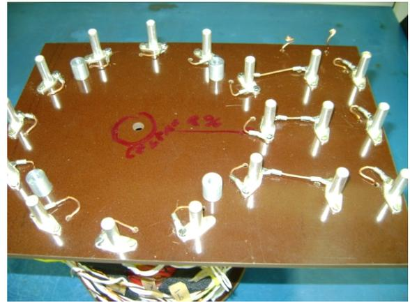
Figure 13. Coaxial output sockets (BPO connectors).
