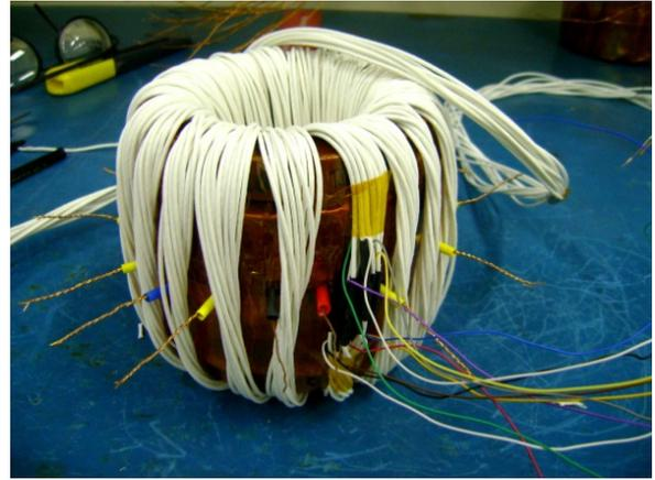
Figure 9. Ratio winding (rope arrangement).
