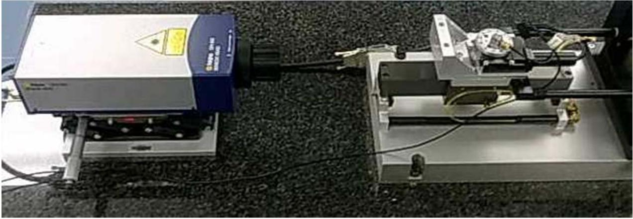
Figure 4. Turntable mounted on top of air-bearing translation stage.
