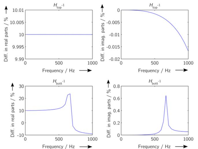
Figure 5. Simulated change of 10% of  $c_T$  of a T10F transducer and its influence on the real and imaginary part of the two frequency response functions function  $H_{\text{top}}$  (top) and  $H_{\text{bott}}$  (bottom), respectively.
