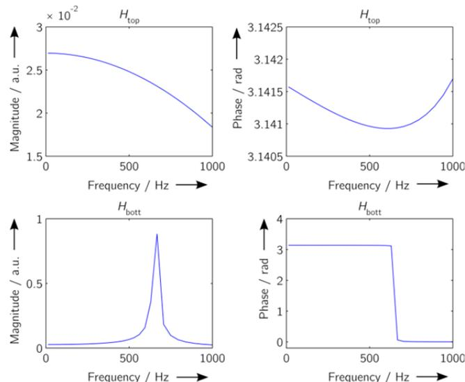
Figure 4. Simulated transfer function  $H_{\text{top}}$  (top) and  $H_{\text{bott}}$  (bottom) calculated with the parameters of an HBM T10F transducer.
