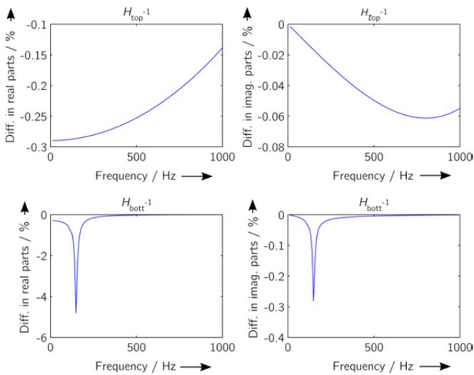
Figure 6. Simulated variation of 10 % of  $J_H$  of a T5 transducer and its influence on the real and imaginary parts of the two frequency response functions.
