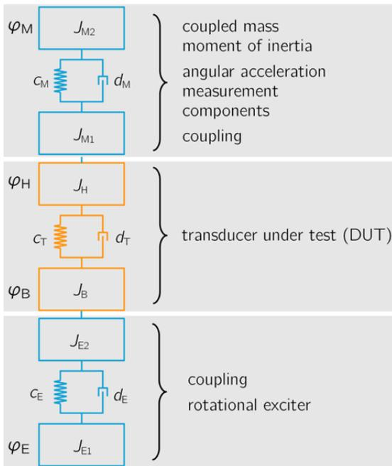
Figure 1. Model of the dynamic torque calibration device (marked in blue) including the transducer under test (marked in orange).
