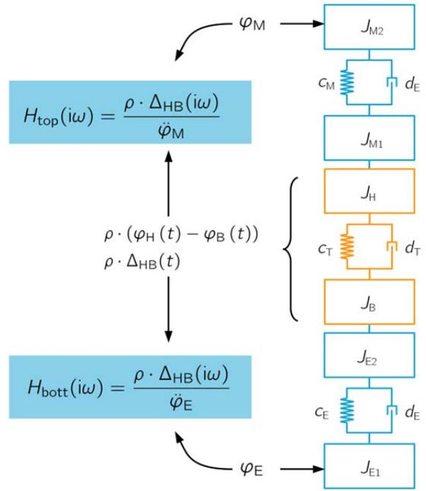
Figure 3. Transfer function based on the acquired measurement channels.
