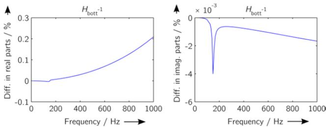
Figure 7. Simulated change of 10 % of  $J_B$  of a T5 transducer and its only very small influence on the real and imaginary part  $H_{bott}$  (bottom).
