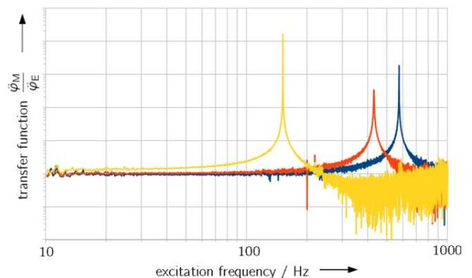
Figure 2. Frequency response of the measuring device with three DUTs of different torsional stiffness and MMOI measured with random noise excitation.
