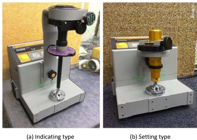
Figure 7. Hand torque screwdrivers (HTDs) installed on the torque screwdriver tester (TDT).
