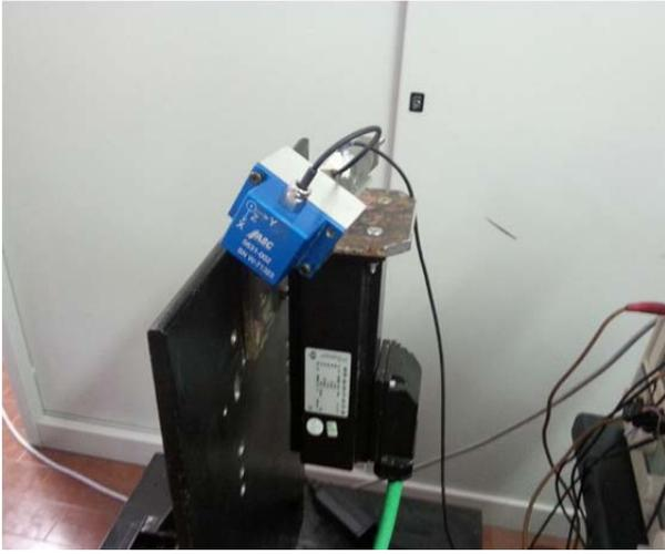
Figure 1. The rotary table, driven by the brushless motor. Rotation angle is measured by a high accuracy angular encoder.
