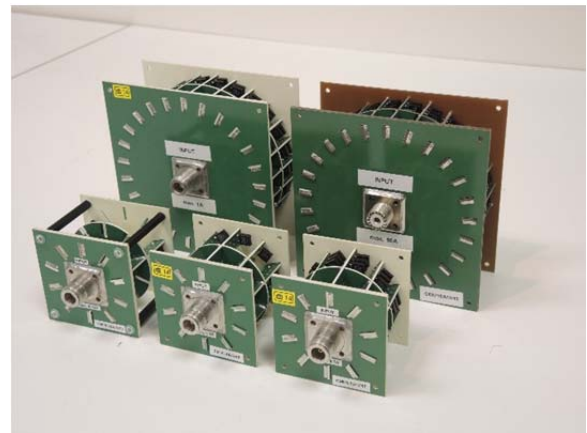
Figure 10. The new generation of cage-type shunts.
