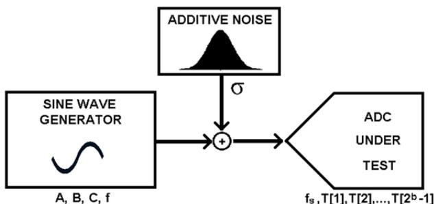
Figure 7. Measurement setup for ADC testing.
