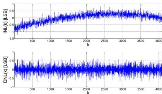
Figure 12. ADC INL and DNL characteristics.
