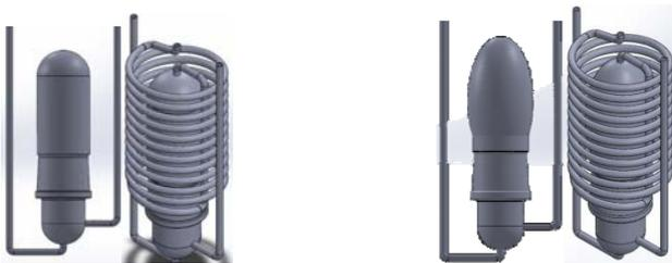
Figure 1. Combustion chamber published in the literature, left side. Combustion chamber from this work, right side.
