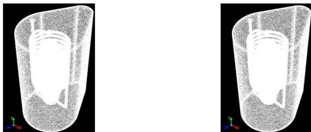
Figure 2. Discretization of calorimeter with burner, heat exchanger and combustion chamber. Right side this work with 1 403 244 nodes; left side from literature with 1 133 433 nodes.
