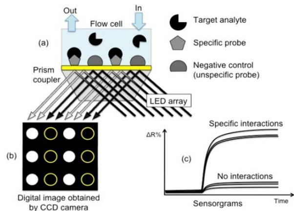
Figure 2. SPRi technology. The receptor is immobilized on the sensor chip gold surface while the ligand is added in solution. From the interaction, a change in the signal is recorded, in label free and real time mode. Parallel analysis on different spots can be performed. The image analysis also visualizes changes on the different spots, providing spatial resolution to the sensorgram changes.
