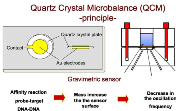
Figure 3. Quartz Crystal Microbalance (QCM): the crystal is sandwiched between two gold electrodes, on which the receptors are immobilized (left). The sensor is inserted in the measuring cell able to operate in static or flow mode (right).
