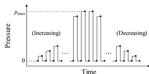
Figure 1. Pressurization procedure for pressure gauge calibration. (a) Stepwise pressurization, (b) 0-A-0 pressurization.
