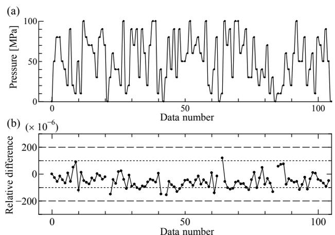
Figure 6. Demonstration experiment with random pressure sequence. (a) Sequence of measurement points, (b) difference between the results obtained with Methods I and II (Method II - Method I).
