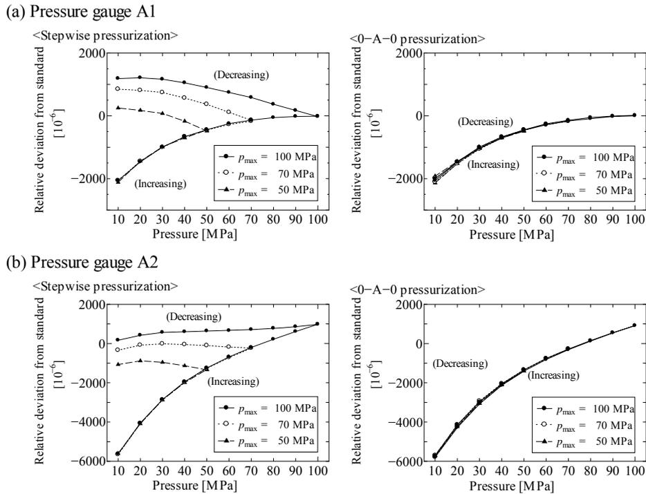
Figure 3. Calibration results for two clamped thin-film pressure sensors with maximum pressures of 50 MPa, 70 MPa, or 100 MPa. (a) Pressure gauge A1, (b) pressure gauge A2. Results for stepwise and 0-A-0 pressurization procedures are compared.
