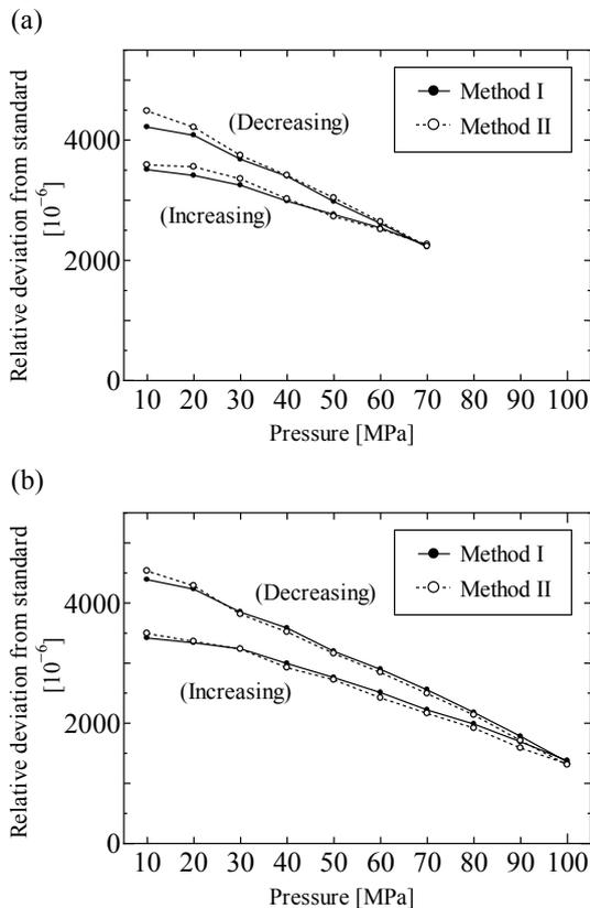
Figure 5. Calibration results for the demonstration experiment with stepwise pressurization for  $p_{max}$  of (a) 70 MPa and (b) 100 MPa.
