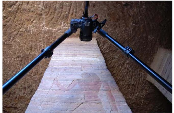
Figure 4. Acquisition step performed with a Canon 5D Mark II and Canon 60D mounted on a tripod half a meter from the surface.
