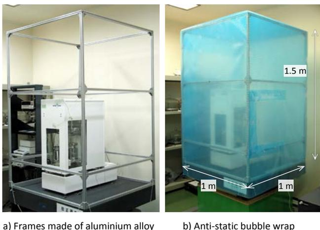
a) Frames made of aluminium alloy      b) Anti-static bubble wrap
