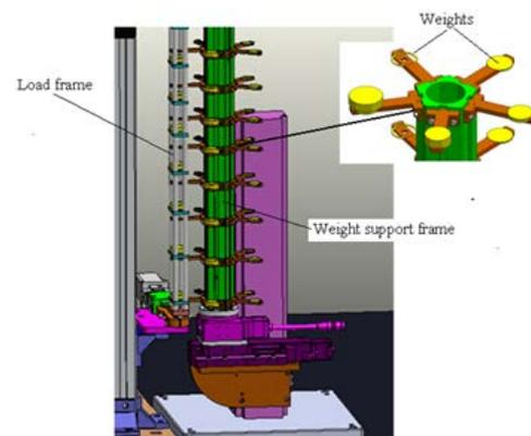
Figure 2. Weight loading system.
