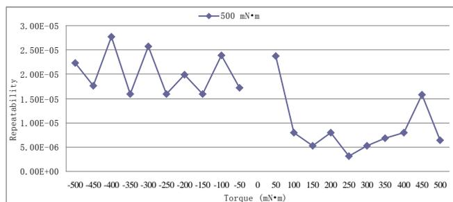
Figure 4. The results of the repeatability test in the  $500 \text{ mN}\cdot\text{m}$  torque range segment.
