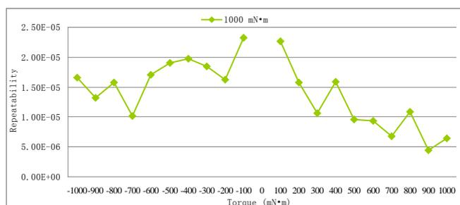
Figure 3. The results of the repeatability test in the  $1 \text{ N}\cdot\text{m}$  torque range segment.
