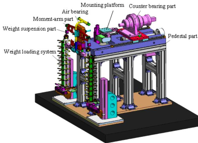
Figure 1. Mechanical structure of the 1 N·m torque standard machine.
