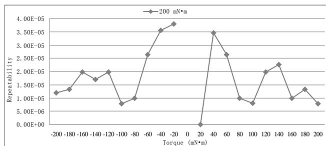
Figure 5. The results of the repeatability test in the  $200 \text{ mN}\cdot\text{m}$  torque range segment.
