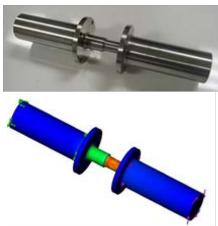
Figure 1. Prototype of the 50 N-m torque transducer with check standard combination.
