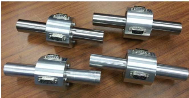
Figure 4. Fabricated torque transducer with check standard combination.
