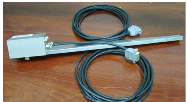
Figure 9. The prototype of the torque transfer wrench with check standard combination.
