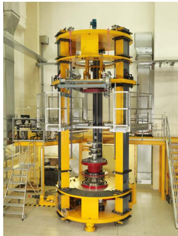
Figure 3. Standard Torque Calibration Machine for nominal torques up to 1.1 MN·m.
