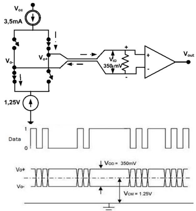
Figure 6. The configuration and signals in the LVDS interface lines [11].
