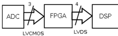
Figure 7. ADC and DSP interface buses in the measurement track.
