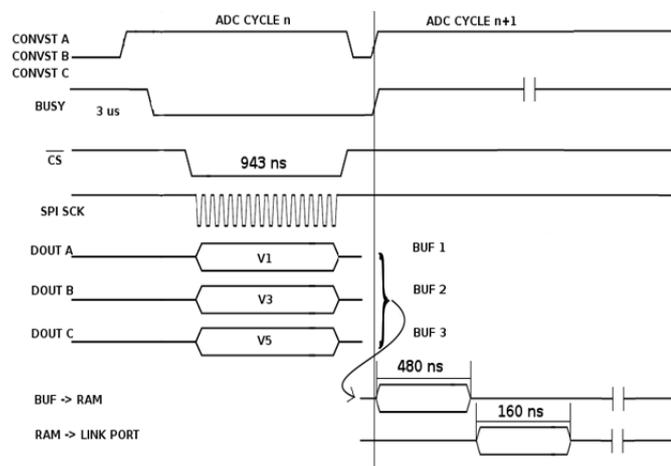
Figure 8. ADC data handling during A/D conversion.
