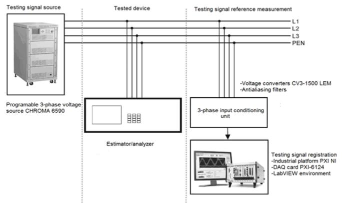
Figure 13. Laboratory stand for experimental verification of the elaborated estimator/analyzer of power quality (version 2.0) based on the appropriately defined testing signals – voltage quality parameters.
