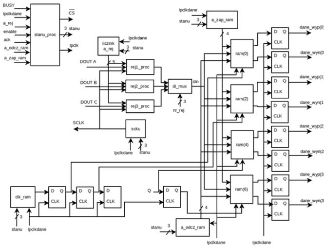
Figure 10. The structure of the functional blocks configured in the FPGA.
