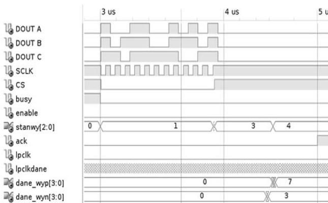
Figure 11. The simulations in the WebPACK environment.
