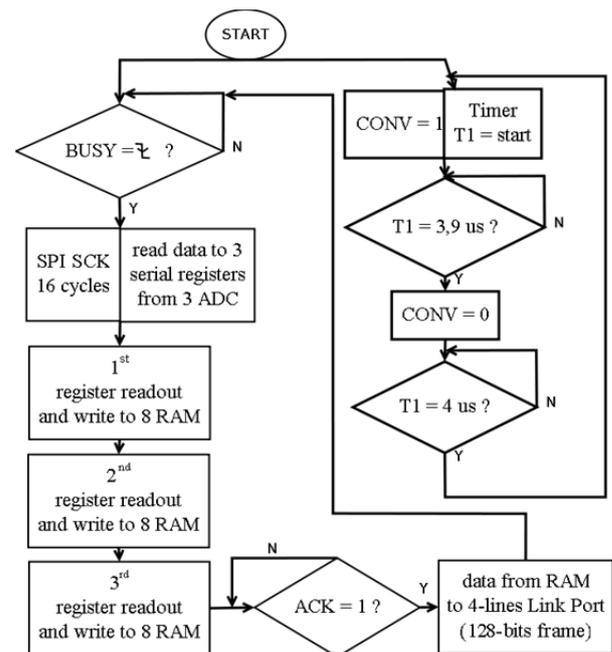
Figure 9. Algorithms performed in the FPGA.
