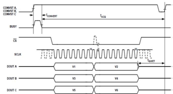
Figure 5. The signals in the AD7656 serial interface lines [8].
