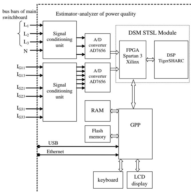
Figure 1. The measurement channels configuration of the developed estimator/analizer.
