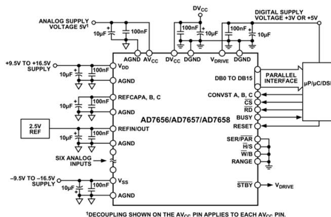
Figure 2. The configuration of AD7656 [8].
