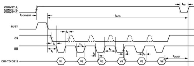
Figure 3. The ADC registers data output procedures through the parallel interface [8].
