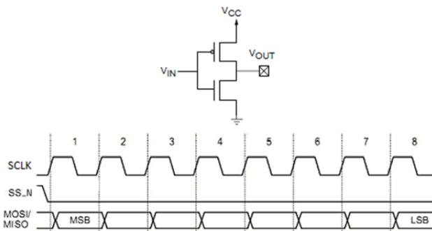
Figure 4. The line driver and waveforms in the SPI interface lines.
