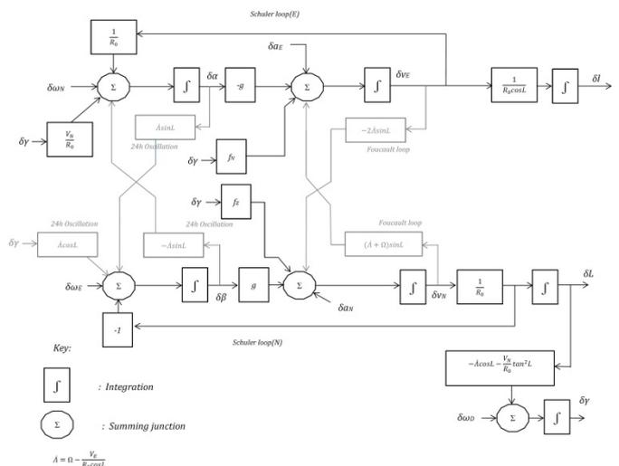
Figure 13. INS long period errors correction block scheme.
