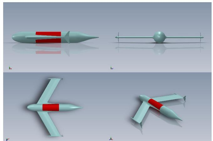
Figure 1. SQUID TUG (Tailless Underwater Glider) view.
