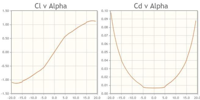
Figure 8. Eppler E838 Hydrofoil characteristics ( $Re = 10^6$ ).
