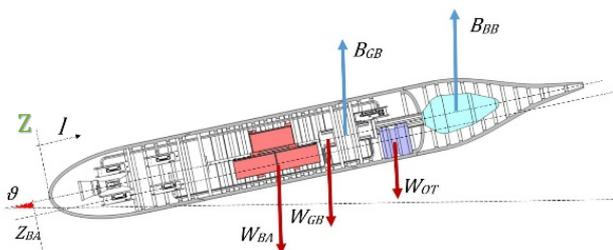
Figure 4. Pitch balance diagram.
