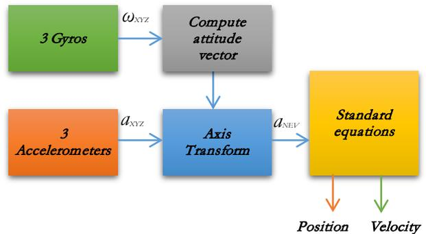
Figure 12. Strapdown INS unit block diagram.
