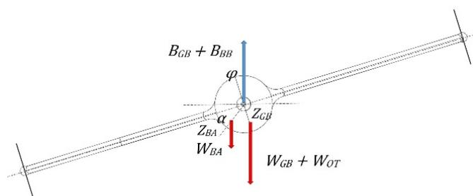
Figure 5. Roll forces balance.
