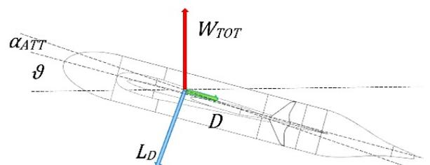
Figure 7. Dynamic vertical forces balance (immersion (top) and emersion (bottom) phases).
