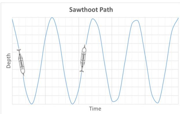
Figure 9. Sawtooth typical glide path (qualitative).
