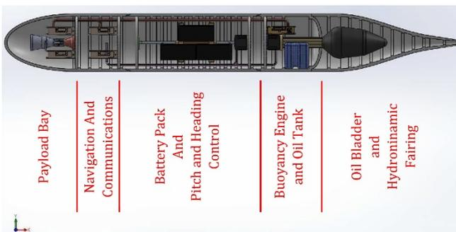
Figure 2. Fuselage profile view (cutaway).
