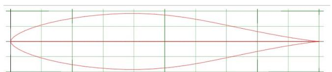
Figure 3. The *Eppler E838 Hydrofoil* profile.
