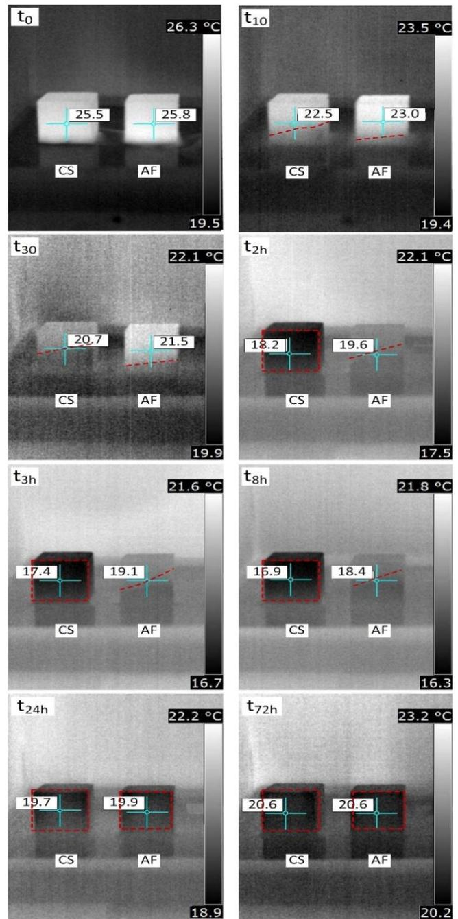
Figure 4. IRT thermal images taken during the capillary water absorption test along the Z direction of San Lucido calcarenite (CS) and Fuscaldó sandstone (AF).
