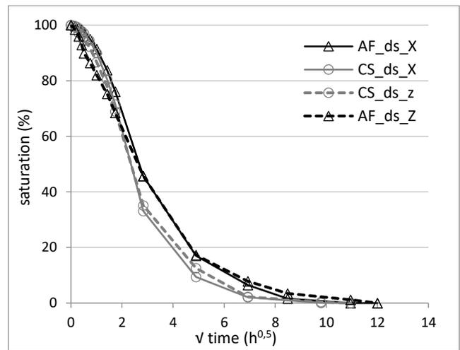
Figure 2. Water desorption curves. Saturation (%) vs. square root of the time ( $\text{h}^{0.5}$ ) along the two investigated directions (X and Z).
