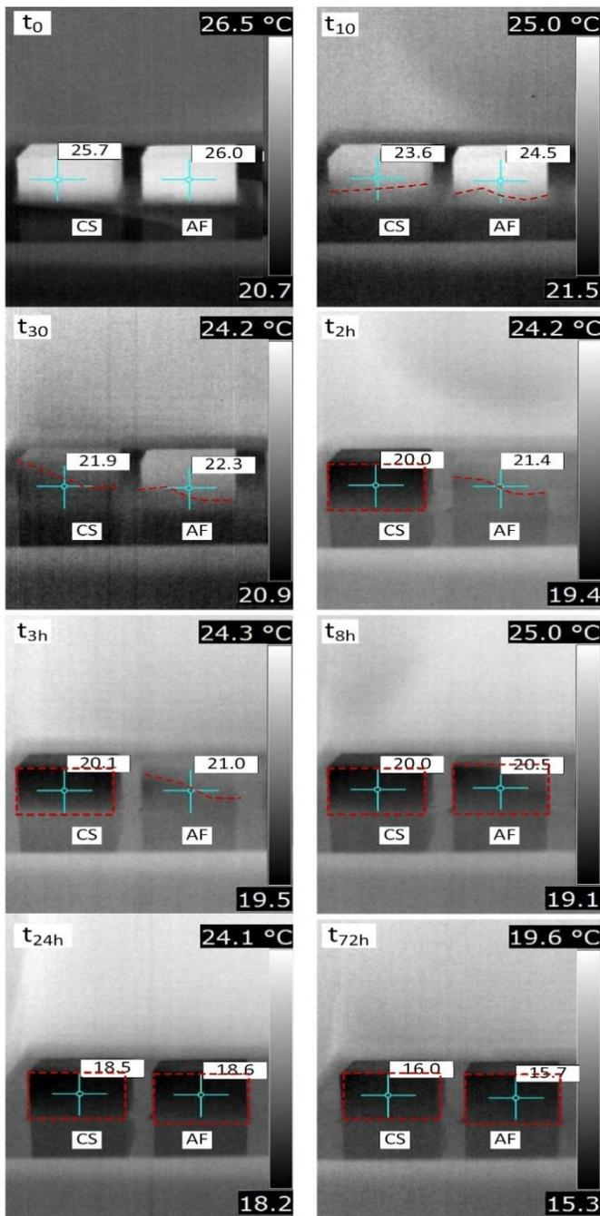
Figure 3. IRT thermal images taken during the capillary water absorption test along the X direction of San Lucido calcarenite (CS) and Fuscaldó sandstone (AF).
