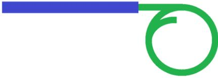
Figure 1. Schematic diagram of the acoustic thermometer with a single waveguide.
