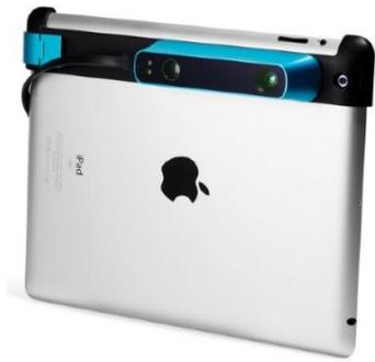
Figure 7. Structure Sensor clipped onto an iPad.
