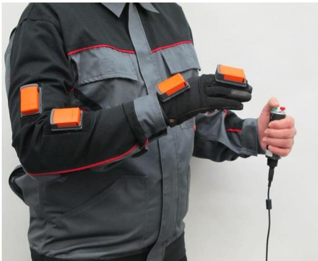
Figure 3. A user wearing the jacket with IMUs attached to it and holding a serial device. The green button is used to start the gesture recognition and the red button is used to stop recognizing gestures.
