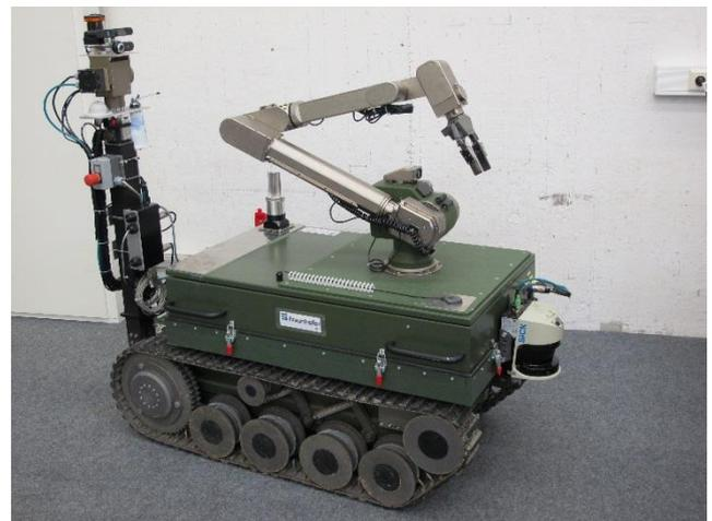
Figure 6. The robot hardware used for demonstrating the gesture-based control.
