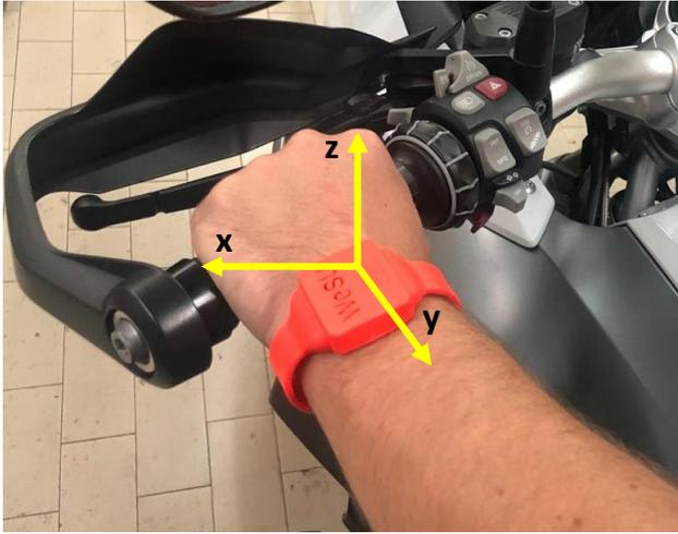
Figure 2. The reference system for the wearable device.
