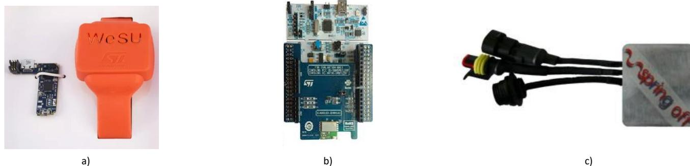
Figure 1. The measurement setup: a) The wearable device, b) The Nucleo board equipped with the Bluetooth module c) The data logger.
