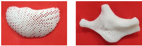
Figure 9. Customised PCL/HA scaffolds for mandibular defect regeneration (i.e., symphysis – left, ramus – right).
