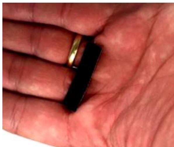
Figure 4. The realised device (length 35 mm, width 11 mm, and thickness about 0.25 mm) with the two electrical contacts on the top and bottom faces. The black surface is the PEDOT:PSS layer. The BC-IL composite is sandwiched between the two PEDOT:PSS layers.
