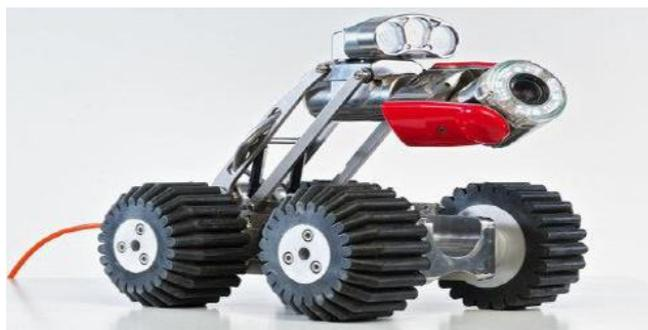
Figure 1. Remotely controlled CCTV camera used in drain and sewer systems inspections [14].
