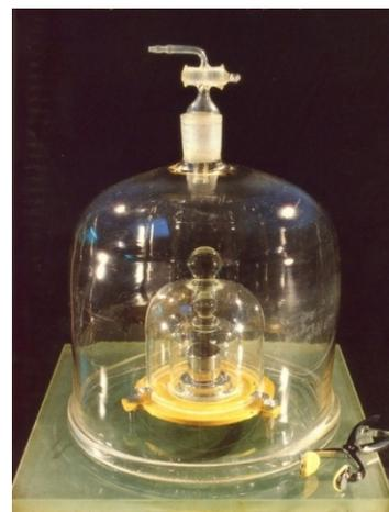
Figure 3. The IPK is kept at the BIPM in Sèvres. It still defines the unit of mass, the kilogram. Its mass,  $m_{\text{IPK}}$ , is defined to be exactly 1 kg with zero uncertainty. In the proposed new SI it will have non-zero uncertainty (source: BIPM, Sèvres, France).
