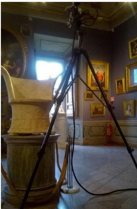
Figure 7. Structured light scanner instrument.
