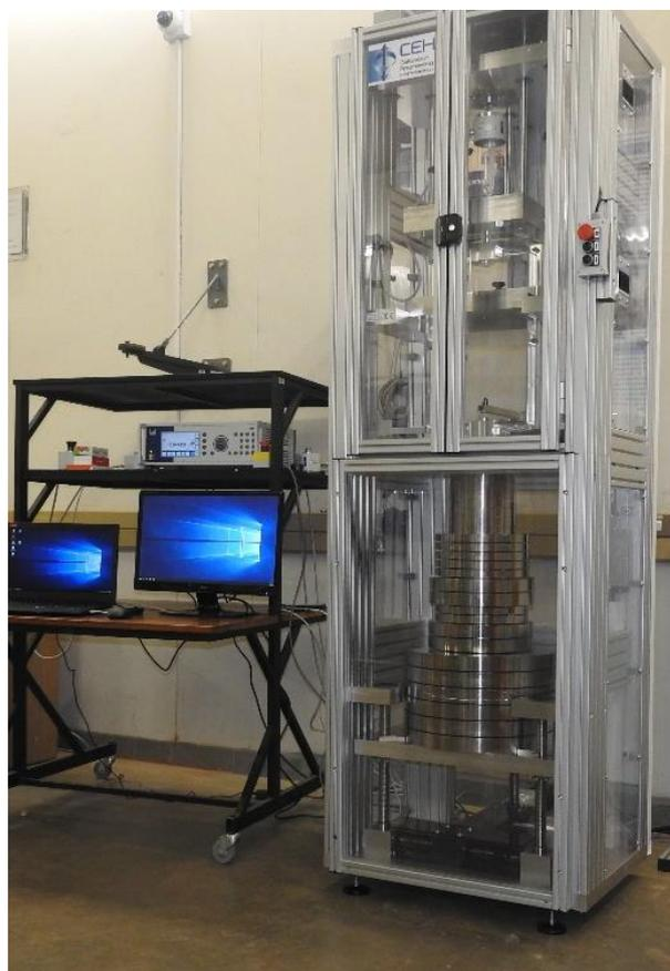
Figure 1: The 5 kN deadweight FSM at NMISA
